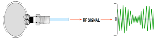
Figure 6. Returned RF signal at vibrating shaft
