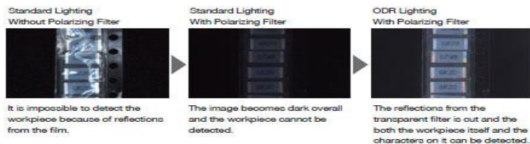
Figure5: Comparison between old system and new system
