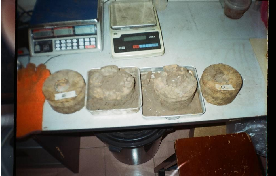
Figure 4. Intactness and uniformity comparison between treated peat CBR samples having fibres with samples without fibres (inside dishes)
