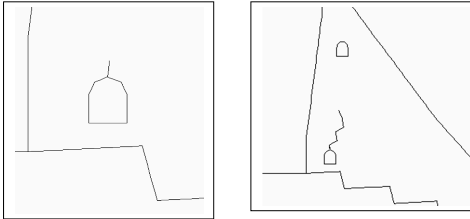
Fig. 12- Propagation of crack No.6 (earthquake load in empty reservoir)
