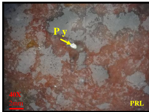
Fig 5: The high contamination of iron oxide leads the red color of matrix. It could be related to presence of jasperoid in this area.
