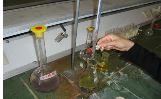
Fig2. Measurement of chloride ion percentage in the sample by using the Potentiometric
