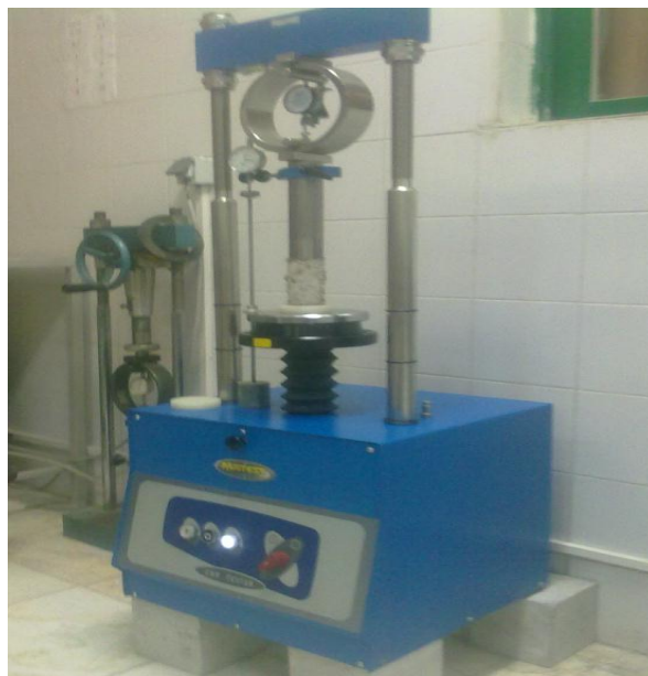
Fig 2: device of Unconfined Compression Test
